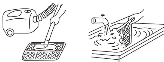
⚠ Don't use hot water over 50°C. It may deform the air filter.
